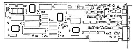
(i)Align the card edge connector over the connector slot and push the LAPC-I board into the slot. Secure the board into the slot with the retaining screw.
