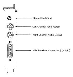
①Connect the MIDI connector box MCB-1 to the MIDI interface Connector. This box provides the connectors for attaching MIDI equipped keyboards and other devices to the LAPC-I card. This box also contains a metronome beeper.
